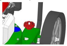
**FOR MAXIMUM PICKUP:** Adjust nozzle close to debris, but without blocking airflow into the nozzle. *NOTE*: Never bury nozzle into debris.
