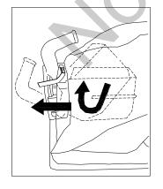
Insert the quick disconnect from the inside of the bag, tilt the handle so it can be fed through first. Then slide the connecting end through and tighten the strap
