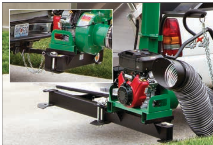
Optional CustomFit™ swing away hitch is mountable to a class III trailer hitch and locks at 90 and 180 degrees so the unit can be swung away. For easy dumping. DL1302, DL1402 and DL1802 models only. (Part No. SAH34)
