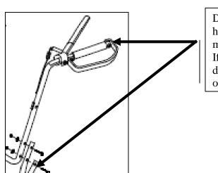
Distance between the back of the handle and the center of the lower mount bolt should be 19 ¼ inches. If less than 19 ¼ the handle is bent down and will require straightening or replacement.
