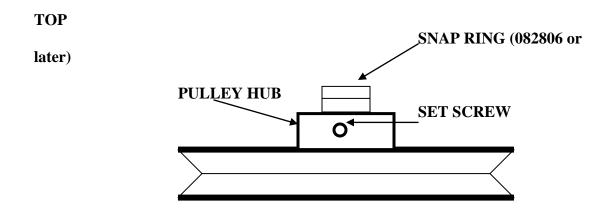
NOTE; Units with serial numbers 082806XXX or later will have a snap ring securing the pulley to the shaft instead of the setscrew.
