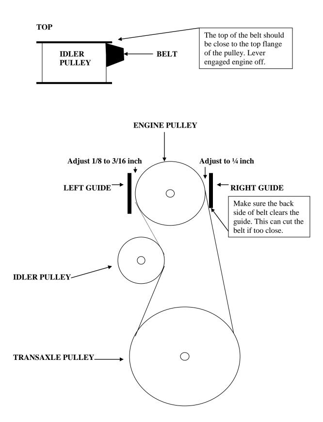
This illustration shows the proper configuration of the drive pulley on the transaxle.
