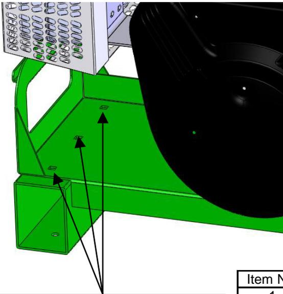
Attach the hanging brackets to the base with the hardware here
