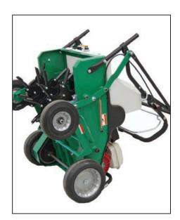
**Tilt up serviceability,** plus Fold-n-Go $^{\text{TM}}$  handles are excellent for transport and fold without tools.
