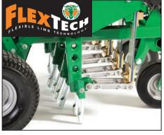
Independently acting, "FLEXTECH" arms are durable and forgiving for unmatched reliability! Reciprocating action drives plug depths up to 2x that of drums. Significantly reduces call backs and/or rework regardless of soil conditions. Patent Pending.
