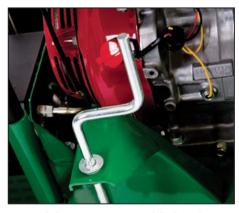
**Powerful suction at variable heights** Readily adjust height from ½" to 3" to accommodate any hard surface needs.
