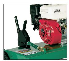
**Infinite, heavy-duty depth adjustments** save on blade wear when compared to preset adjustments that may promote premature flail wear.
