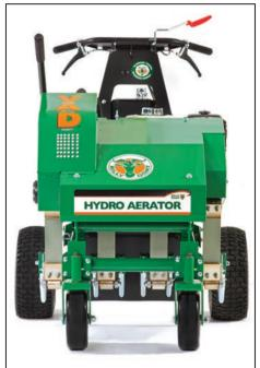
**30"** wide aerating productivity is combined with outstanding durability, speed, deep plug depth and no need to double aerate! This machine fits everywhere you need to go. No need for both large and small machines.
