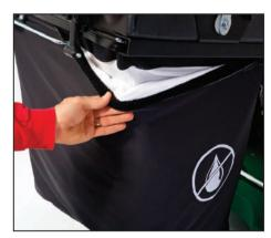
**Optional electrostatic dust sock kit** traps dust for optimum operator and air quality protection. (Part No. 80023248)
