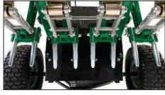
**Fast tine service** Only 8 tines and 4 bolts which are easily accessed and takes 10% of the time needed to service 40+ tine, 2-bolt drum units.
