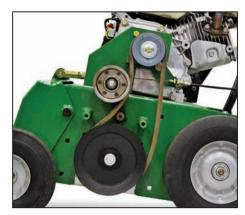
**Premium pulleys,** easy to adjust idler, and easy to change belt contribute to simple service and long life. Protected by a steel guard.
