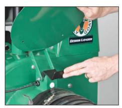
**Safety kill switch** Quick connect / release hose clamp with safety interlock.
