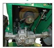
Tuff Torq™ hydrostatic transaxle with ETC (Enhanced Traction Control) is fully automatic, sensing when the rear wheel starts to spin, locking the wheel and giving it positive traction. Provides superior traction on hills or in wet and uneven conditions.
