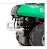
Heavy Duty Bumpers The wide front and rear bumpers protect the rider against accidental impacts and incorporates tie-down points for securing the machine during transportation.
