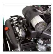
Transmission Oil Cooler A remote transmission oil cooler controls the transmission oil temperature even in the toughest conditions, reducing thermal oil breakdown for an extended operating life of the system.
