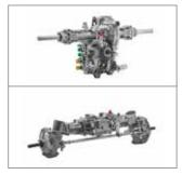
Drive System The Tuff Torq<sup>™</sup> 4WD system automatically controls the output to all drive wheels. Combined with a manual locking differential, this 4WD system provides all the traction you need in challenging terrain.
