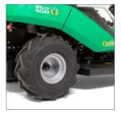
Drive Wheels Large drive wheels with agricultural tread ensure sufficient grip. The pivoting front axle allows all four driven wheels to remain in contact with the ground for maximum traction.
