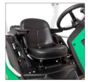
Ergonomic Operators Platform The large operators platform provides sufficient space for even the tallest user. Secundairy footrests provide a secure foothold expecially for use on hillsides. The contoured seat with armrests keeps you comfortable all day and is equipped with fore and aft positioning. Integrated hand rails provide a secure grip on the machine when needed.
