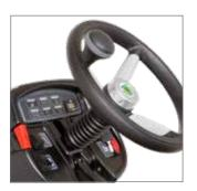
User Friendly Dashboard The operators compartment features a dashboard with control and warning lights, electric PTO engagement switch with soft start function, steering wheel with tilt-function and spinner knob, cruise control switch and a parking-brake lever.
