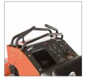
Quad Control Handle System™ This system offers seamless forward/ reverse direction, automatic return to neutral, integrated operator presence control and a self-activating parking brake. Intuitive controls for ease of operation.
