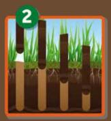
The vertical motion of a tine removes small plugs of soil from the ground.
