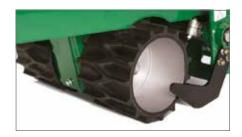
Unique Paddle-Style Drive Wheels SC181HEU model. For landscape applications. Designed to shed mud in wet conditions and grip in dry for improved cutting in all conditions.
