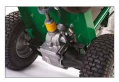
$\label{eq:hydrostatic} Hydrostatic \ Drive \ Transmission$  The self propelled models have a hydrostatic transmission from 0 ~ 4,8 km/h with infinite forward and reverse.
