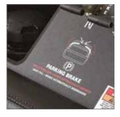
Automatic Parking Brake The Hurricane™ blowers automatically engage an internal parking brake any time the operator leaves the platform.
