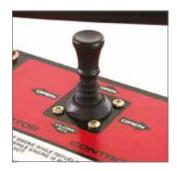
Joystick Deflector Control The joystick allows the operator full control of the air flow direction, from left, right or forward directions. Pulling back on the joystick closes all deflectors for transport.
