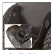
Front & Rear Tie Downs Convenient tie-down points make machine transport safe.
