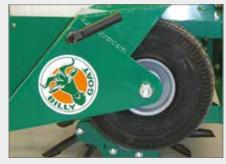
**Tine Engagement Bar and Footpad**Engage tines by stepping on the footpad. Disengage by pulling out the spring loaded lever.
