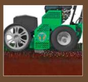
The seeds fall into the soil grooves made by the rotor blades and then pushed deep into the blade passage.
