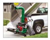
CustomFit<sup>™</sup> Swing Away Hitch Locks at 90° and 180° so the unit can be swung away for easy dumping. (SAH34)
