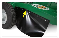
Long reach front end is angled down Longer frame is angled toward the cutter head for longer reach and better grinding versus others on the market.
