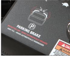
**Automatic parking brake** self-activates if the need to briefly step off of the machine arises. (X3000, Z3000)
