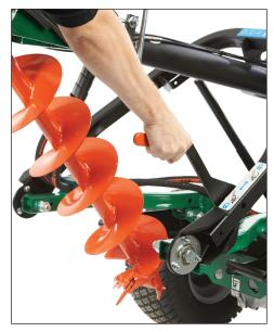
Auger bit position during transport and drill For efficient, compact transport, bit locks in forward position and easily clears the ground for simple moving hole-to-hole. Unlock both the transport handle and pull the quick release pin to swing the bit into position for vertical drilling.
