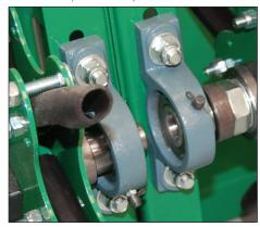
**Pillow block bearings** with grease zerks reduce wear and downtime for maintenance.
