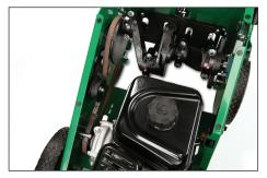
Longer belt span improves belt de-clutching and increases belt life. (PL1801H & PL1803V)
