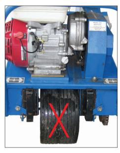
The outboard drive wheels eliminate both center wheel slip and damage from ramp loading with the tines engaged.
