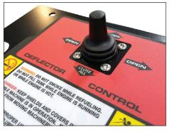
Joy stick deflector control with improved mounting bezel allows for quick and easy control of air flow from left, right or forward directions, eliminating the need to blow in reverse. Simply pull-back on the lever to close flow for transport. (X3000, Z3000)
