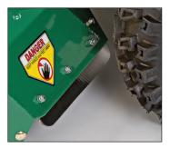
**Rubberized rear deck trim** allows for easier stump clearance in reverse.
