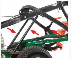
**Gas spring lift struts** assist the operator when lifting the bit from the hole, reducing fatigue.
