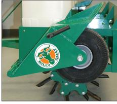
**Tine engagement** Lower and engage the tines by releasing the spring loaded lever. Raise the tines out of the ground by stepping on the footpad in combination with pulling on the provided lift steel bar when inserted into the lift slot.
