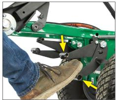
**Spring loaded parking brake** on rear wheels helps stabilize the machine for straight line drilling on uneven or sloped terrain. Bottom pedal engages brake and top pedal disengages brake.
