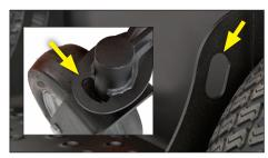
**Front and rear tie downs** offer secure tie down points for ease of transport.
