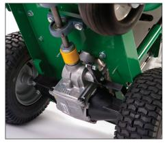
**Hydro-drive transmission** Hydrostatic transmission with infinite forward and reverse speeds, 0-3 mph, and shift on the fly. Negotiate tight spots quickly and with unbelievable ease. (QV550VSP, QV550HSP, QV900HSP models)
