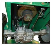
Tuff Torq" hydrostatic transaxle with ETC (Enhanced Traction Control) is fully automatic, sensing when the rear wheel starts to spin, locking the wheel and giving it positive traction. Provides superior traction on hills or in wet and uneven conditions.
